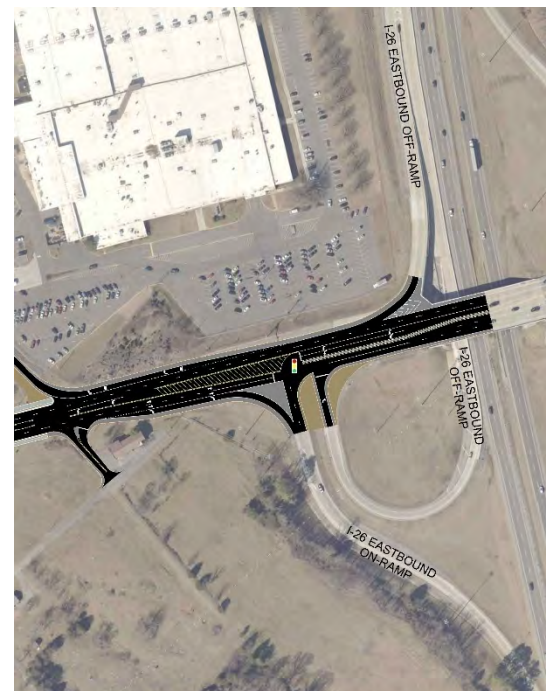
Figure 5-14 Proposed I-26 Eastbound Off-Ramp Reconfiguration
