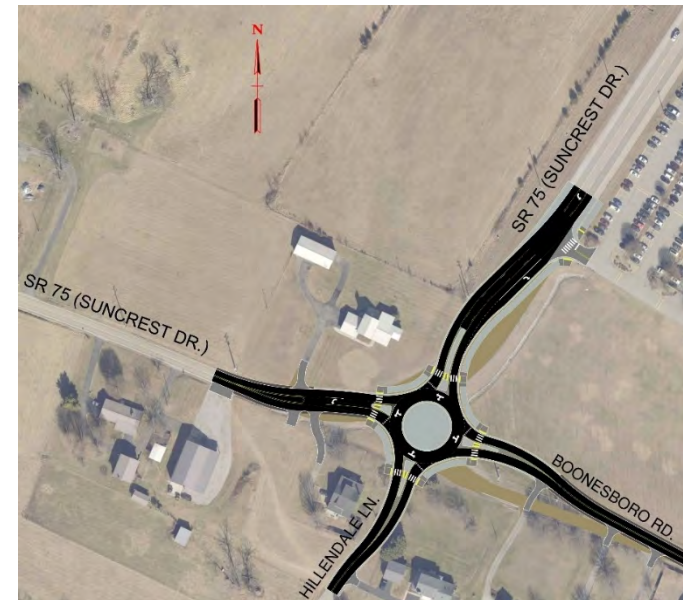
Figure 5-8 Proposed Roundabout at Boonesboro Road/Hillendale Lane
