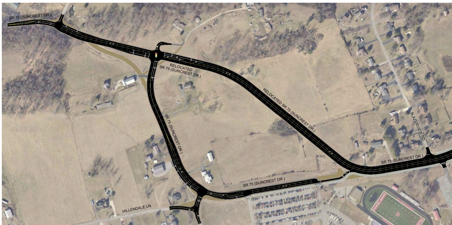
Figure 5-10 Proposed SR 75 (Suncrest Drive) Phase 2 Realignment
