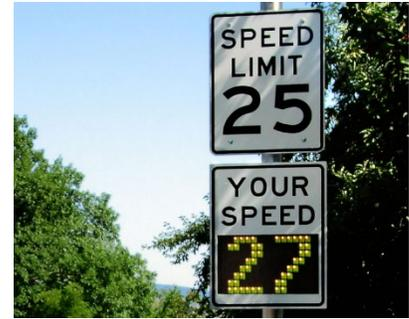
Figure 25: Dynamic speed feedback sign (Source: FHWA)
