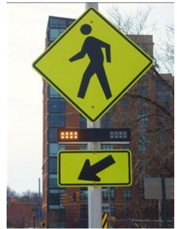
Figure 24: Rectangular Rapid Flashing Beacon (Source: FHWA MUTCD)
