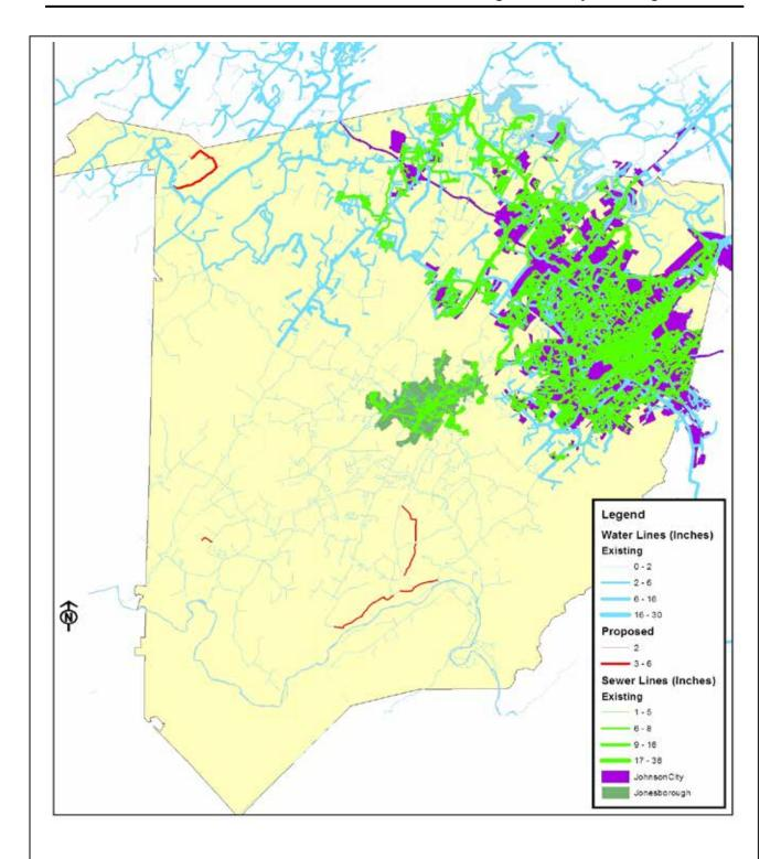
FIGURE 7.4: WATER AND SEWER LINES
