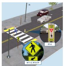
Figure 31: High-visibility crosswalk (Source: FHWA)
