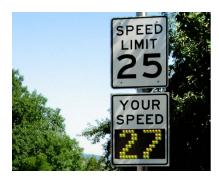
Figure 25: Dynamic speed feedback sign (Source: FHWA)
